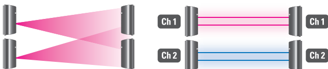
| Conventional beam sensor (Confusion occurs among beams)
